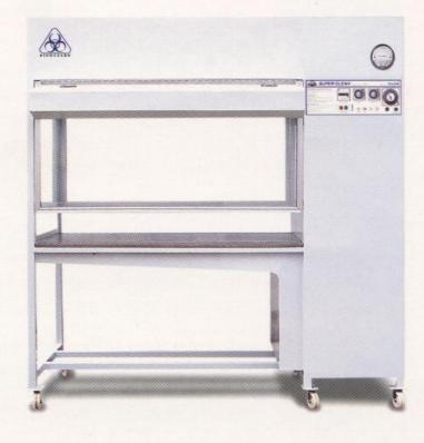
The air flow is vertical drawnflow work station, efficiency protecting the material against contamination. At the same time its offer well defined operator and environment protection against active or dangerous work substances. 20-25% of the recirculated air is exhausted after through the second HEPA-filter.
